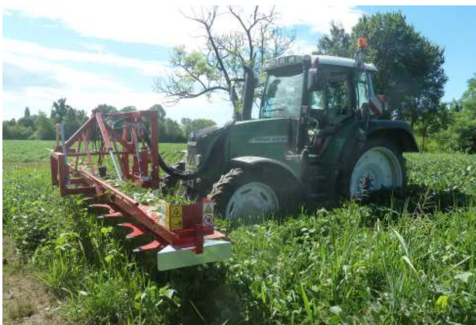
fig.1. Horizontal weed trimmer.
