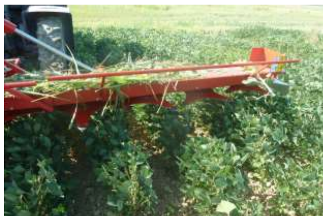
Fig. 4. Weed trimmer cutting knives
