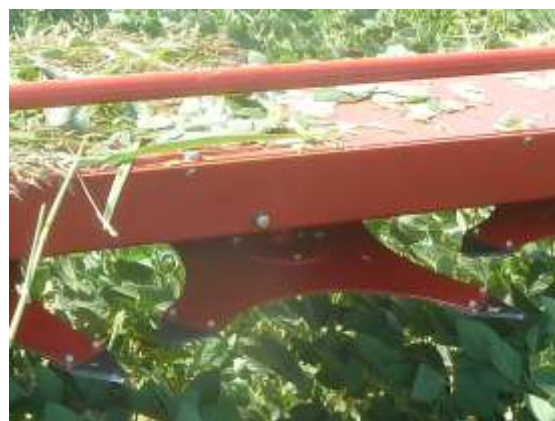
Fig. 5. Weed trimmer cutting knives.
